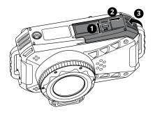
2. While checking the positive and negative of the battery, use the side of the battery to release the battery lock lever in the direction of the arrow to install the battery correctly.
