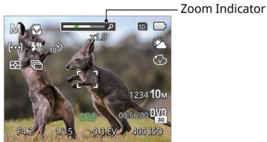
When the Optical Zoom reaches the threshold as Digital Zoom, release and turn the Zoom button to T to switch between the Optical Zoom and Digital Zoom.
